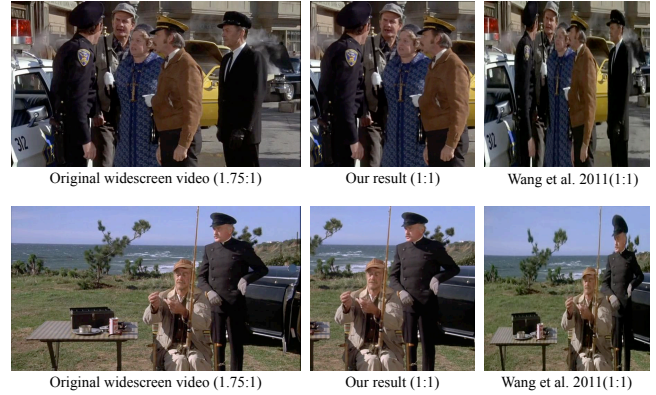
Fig. 7: Sample frames are shown from two example sequences. We compare with the optimized crop and warp method of Wang et al. (2011). Significant distortions are introduced by their method for large scale changes. Images from Herbie Rides Again courtesy The Walt Disney Company.
