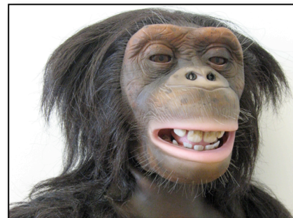
Figure 1. The robot Virgil. It has 18 degrees-of-freedom.
