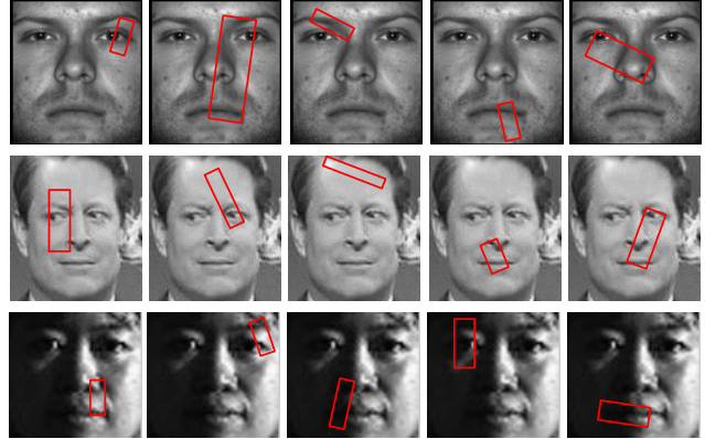
Figure 2. The highest weighted rectangle features obtained after Boosting for Extended Yale B dataset (top), LFW dataset (middle), and CMU PIE dataset(bottom).
