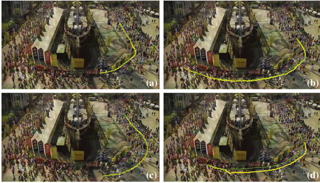
Fig. 11. Qualitative results on Sequence 5: This figure shows tracks of four different individuals from Sequence 5. The ground truth is shown in green, while track from proposed method is in yellow. In (a–c), the track from proposed method perfectly aligns with the ground truth, while (d) shows a failure case, where the track was lost soon after the initialization. (For interpretation of the references to color in this figure legend, the reader is referred to the web version of this article.)
