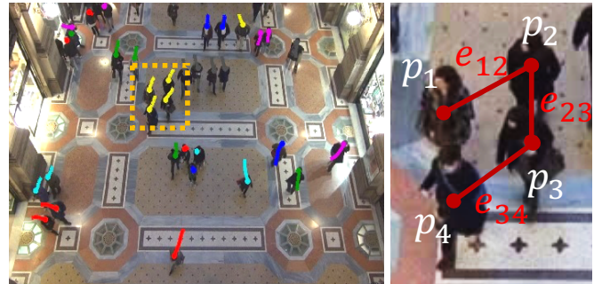
Fig. 5. An example of our minimum spanning tree group structure model. The figure on the left shows the groups found in frame 638 of Galleria1 sequence (nearby tracks with similar color correspond to one group). The figure on the right illustrates the model created for the group inside the yellow box. p_i denotes the location of the target and e_{ij} denotes the relative distance between the two targets i and j .
