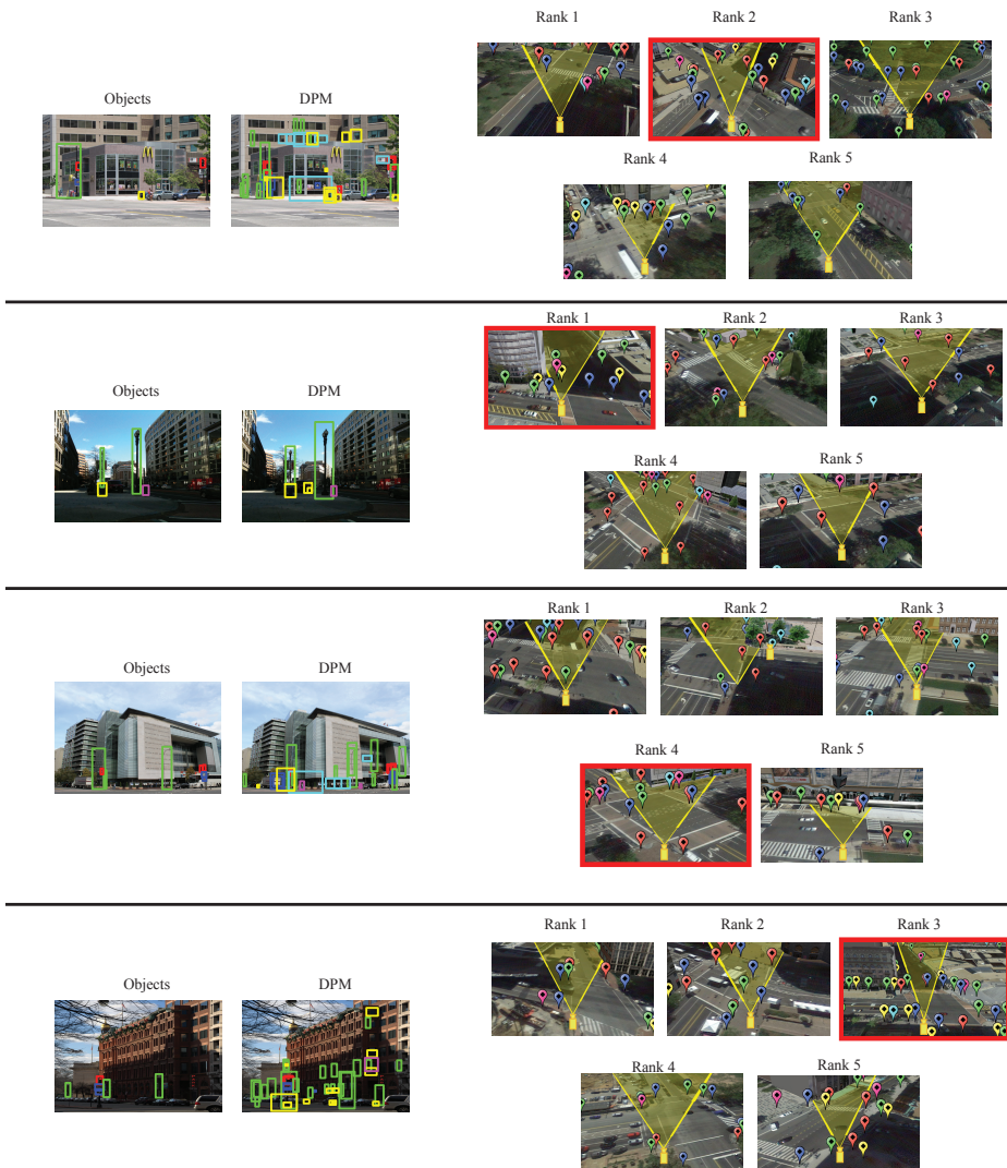
Fig. 8. Sample geo-localization results for four query images from Panoramio and Flickr. The images corresponding to the five best matching locations as well as the DPM detections and the ground truth objects are shown. The image corresponding to the correct location (i.e., the grid point within 20m of the ground truth GPS location.) is marked with the red boundary. As apparent in the figure, the correct location is among the best matching geo-locations as a results of the similarity between the objects visible in the image and the GIS database of the ground truth location.
