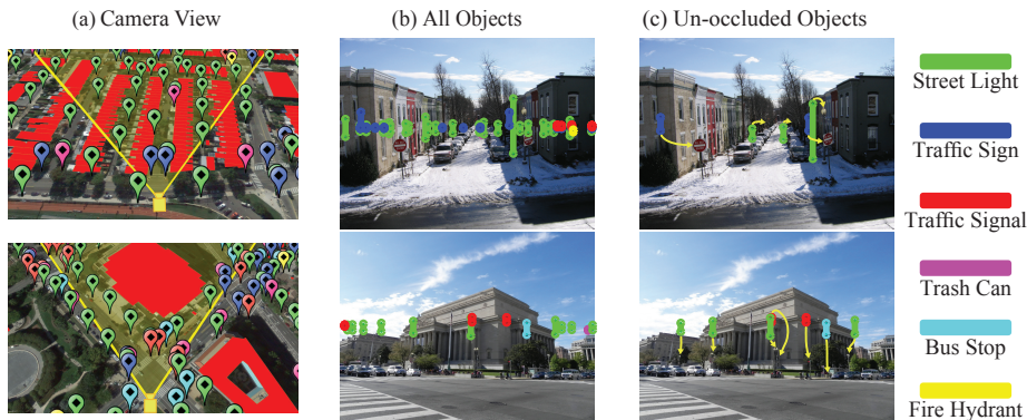
Fig. 1. The process of acquiring GIS projections for two sample images. Part (a) illustrates the camera view (yellow lines) shown in the overhead view with the occlusion segments (red) and GIS objects. Part (b) shows the projections prior to occlusion handling. Part (c) shows the final projections after occlusion handling along with their corresponding objects.
