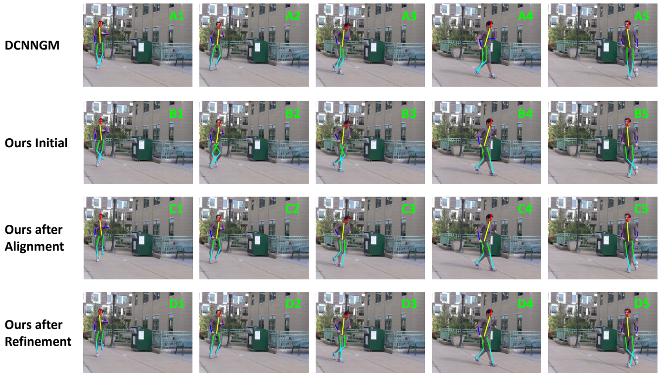
Fig. 9. An Illustration for Limb Alignments and Refinements. “DCNNGM” shows the initial pose estimation; “Ours Initial” shows the results after “Abstraction” and “Association”; “Ours after Alignment” and “Ours after Refinement” show the results after these two steps respectively.
