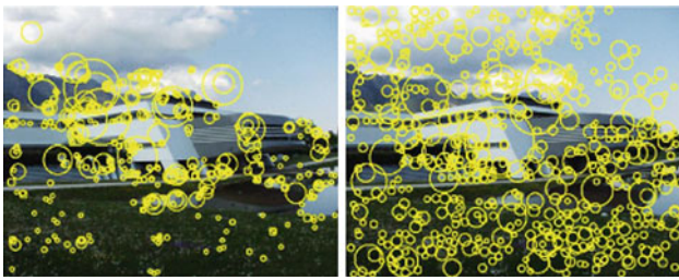
Fig. 3 Example results of local detectors: Harris–Laplace ( left ) and DoG ( right ). The images are obtained from [30]
