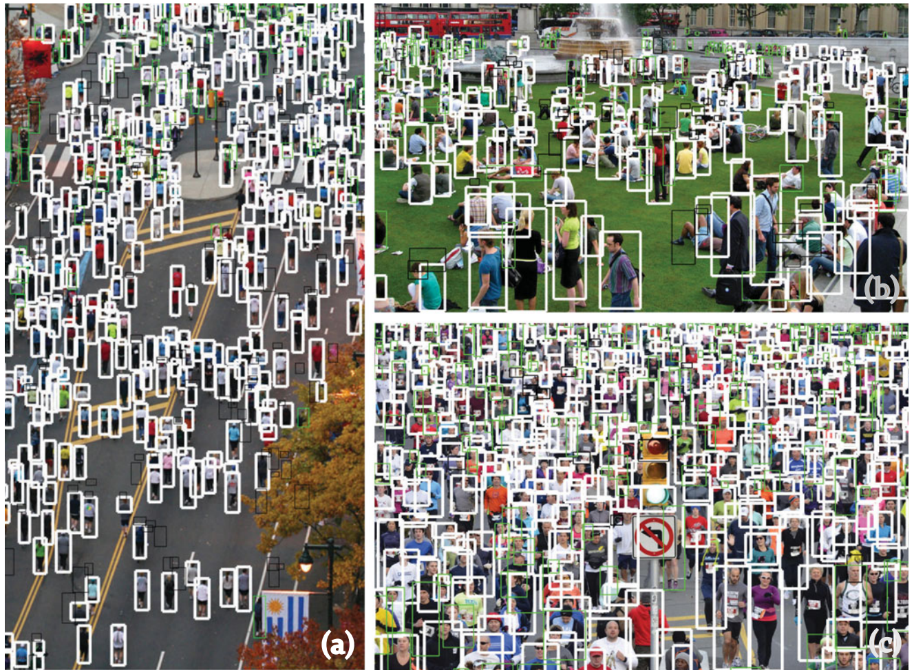
Fig. 13. In this figure, white bounding boxes signify true detections (TP), black boxes indicate false alarms (FP), while green represents miss-detections (FN). In (a), the crowd is sparse with humans inclined at an angle due to camera position. In (b), the humans appear in varied poses, whereas (c) is characterized by severe occlusions. The proposed approach gives excellent results for all three scenarios.
