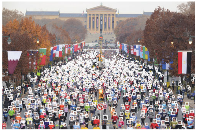
Fig. 6. Results after using scale-consistency and combinations-of-parts detection on an image containing almost 3,000 people. The result is 82 percent precision at 60 percent recall evaluated only on heads. White bounding boxes signify true positives, whereas black represents false positives.
