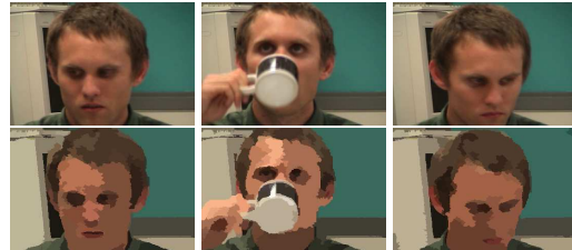
Figure 3: Top row: Sequence showing person drinking from a mug. Bottom row: Mean shift segmentation performed on the above three frames. The idea of this feature is to count the number of segments in each given region. For this example computation the region is the whole image. Frames 2854, 2897, and 2990 are shown.
