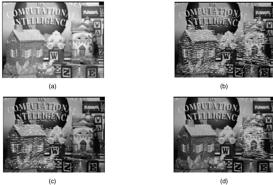
Fig. 3. Results for a sequence with camera and right toy house moving. (a) Frame 1. (b) Measured optical flow field overlay with Frame 1. The vector lengths are scaled by 2.0. (c) Segmentation result for Object 1: the background. (d) Segmentation result for Object 2: the right toy house.
