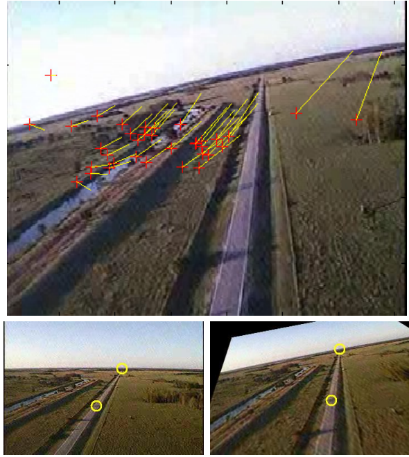
Fig. 8. The result of performing registration between a test frame ( right ) and a reference frame ( left ) is a matrix that can map every point in the reference image to a corresponding coordinate in the landing image, as shown by the warped image ( top ).
