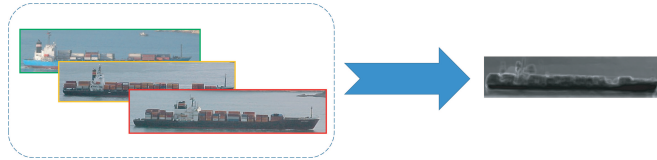
Figure 2. MACH filters combine a collection of training images (left) into a single composite template (right) by optimizing a set of metrics.
