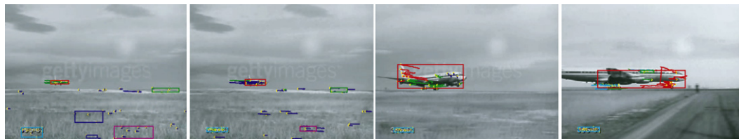
Fig. 13. Note the change in size and viewpoint of the tracked (red label) airplane through the video shot. The extracted volume corresponding to the airplane captures all these different views and can be very useful in matching an airplane with only one of the views. (For interpretation of color mentioned in this figure the reader is referred to the web version of the article.)
