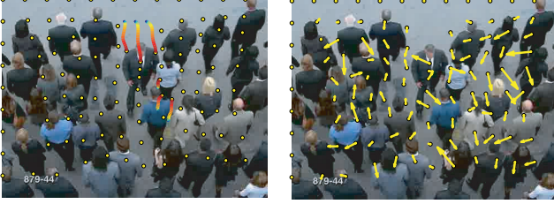
Figure 3. An example of particle advection using the average optical flow field and the corresponding interaction forces. (Left) The trajectories of a small set of particles are depicted for demonstration. (Right) The set of computed interaction forces of particles.
