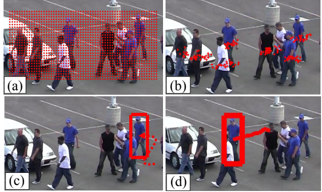
Figure 2: Tracking steps for one person in batch of frames. (a) shows the union of dense candidate windows used in a batch of frames in our method. (b) illustrates the union of human detection results of [15]. (c) shows the most violated constraint found through TINF to update the classifier and in (d) we show the tracking result of our method.
