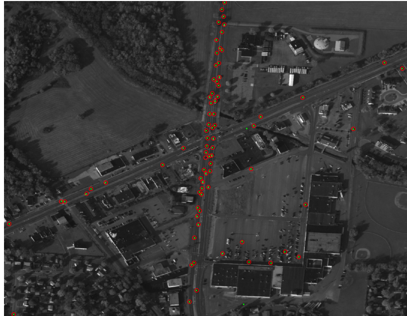
(i) AOI 40 results using 5-frames and the binary segmentation formulation for FoveaNet. ClusterNet output shown at left; FoveaNet output and ground-truth shown at right.
