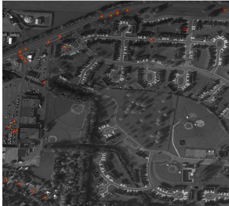
(k) AOI 41 results using 5-frames and the binary segmentation formulation for FoveaNet. ClusterNet output shown at left; FoveaNet output and ground-truth shown at right.
