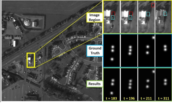
Figure 7: Persistent detection results for AOI 42. The video frame number is marked at the bottom of each column in yellow. Top Row: Yellow-boxed image region at labeled times. In frames 183 – 196, the black car (red-boxed) in the shadow of the building is nearly invisible to the naked eye. In frame 311, due to motion parallax, the white vehicle (teal-boxed) is nearly completely occluded by the building. Middle Row: Ground-truth heatmap. Bottom Row: Output heatmap without any post-processing.
