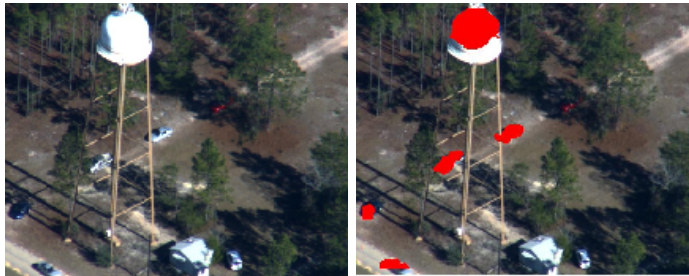
Fig. 1. Illustration of drawbacks of homography based detection approach, where out of plane objects (water tower) are incorrectly detected as moving objects. Left image shows original frames, and right image overlays red detection masks over the images. Detection is performed by image registration followed by background subtraction.
