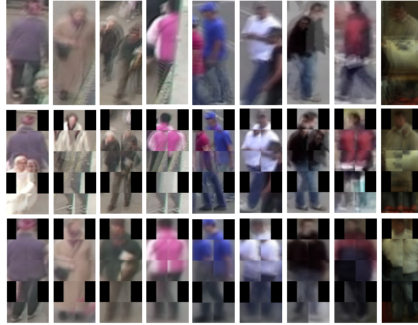
Fig. 3. Three different methods for pedestrian appearance learning. Each figure shows average color of training samples over a short pedestrian tracklet. A simple average over the entire person bounding box is shown in the top row, while the middle row uses detected DPM parts, and our tracked parts are used for examples in the bottom row. Using the entire person bounding box the model is very vague. Since a certain minimum number of parts are always detected in DPM, the model contains background when the person is partially occluded. The handling of occlusion and clutter for parts while temporally aligning them, makes our model more accurate.
