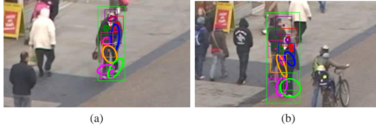
Fig. 2. An illustration of the effect of merged detections on tracking. The figure shows parts of two frames from the Town Center sequence, centered around a target. The large green bounding boxes show the location and scale of pedestrian detection, and the smaller colored bounding boxes show location of parts detections. The similarly colored ellipses represent the online learned model of part locations with respect to the human. In (a), the locations of detected parts are likely as per the model because all parts are within or close to the error ellipses. Figure (b) shows a subsequent frame where two humans are merged into the same detection using the head and shoulders of the incorrect target, thereby producing part detections that are far away from the predicted positions. The initial pedestrian tracklet will therefore be disconnected at this frame.
