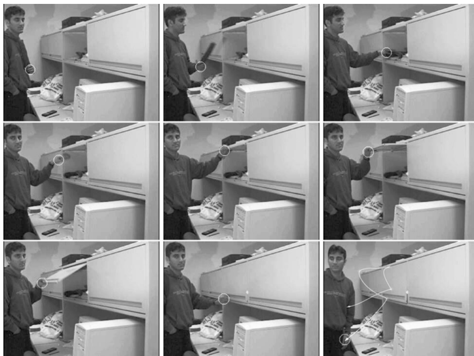
Figure 18. Action 2: Put down the object in the cabinet, then close the door (every 15th frame of the sequence is shown). The hand is highlighted with a white circle, and its trajectory is superimposed on the last frame.
