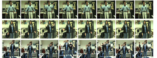
Figure 7: The output of the view invariant dynamic time warping. The columns represent the synchronized corresponding frames. Every 40th of the output frames are shown, they are 11,51,91,131,171,211,251,291.
