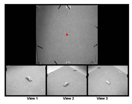
**Figure 3**: The views from the 3 separate nodes (shown at the bottom) are processed locally by an ATD/R, and the position of the target is reported. This data is collected at a central computer where the target coordinates are converted to a common reference frame and fused to depict the location of the target on a site map (or overhead image).
