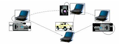
**Figure 2:** Multiple platforms (sensors) are networked to a central computer where ATD/R information is combined into a common reference frame.
