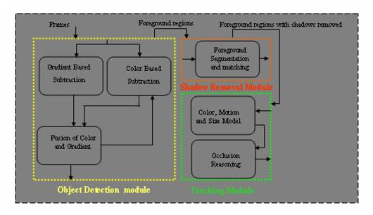
**Figure 4**: A overview of the KNIGHT motion based detection and tracking system for humans and vehicles. Additional details can be found at http://www.cs.ucf.edu/~vision/projects/Knight/Knight.html
