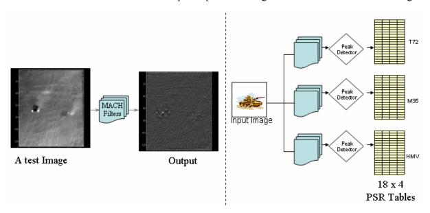
**Figure 1**: An input image is processed by a bank of correlation filters to detect and identify targets. The filter with the highest PSR determines the class of the object, and the position of the correlation peak indicates its location.
