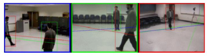
**Figure 5**: The automatic calibration of three separate cameras with overlapping fields of view (FOVs) is shown. The FOV boundary lines are established by observing where moving objects visible in one camera simultaneously appear at the edge of another camera's view. Places where this occur represent points on the boundaries of FOVs of other cameras that are visible in the current view.
