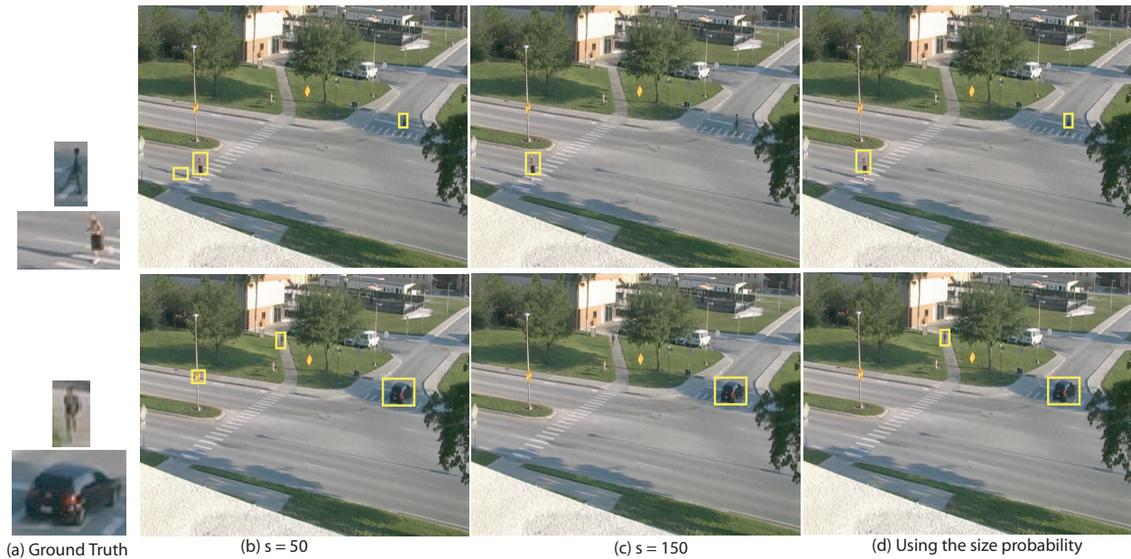
Figure 3.7: Scene 2. Improvement in object detection by the proposed size model. Each row presents an instance in the same video. Column (a) shows the manually extracted patches of the objects currently present in the scene. Column (b) is the output when a uniform global value of s = 50 is used. Noisy foreground blobs are also detected as valid objects (red ellipses). (c) presents output when s = 150 is used throughout the scene. Individuals are not detected (red ellipses) when the object size is small. (d) presents results of the proposed size model. In both scenarios the valid objects are detected and the noisy observations are avoided.
