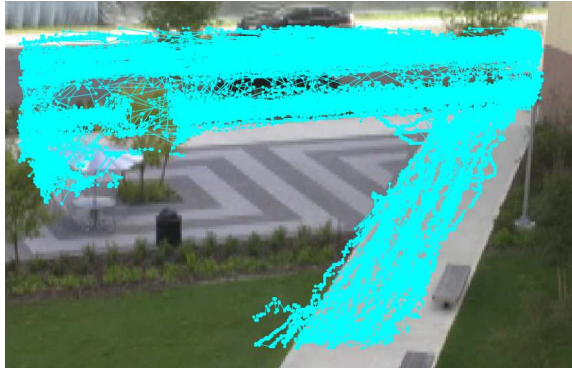
Figure 3.3: A subset of tracks used in the training of the scene model. Multiple transition vectors from each observation contribute towards learning the pdf at that location.
