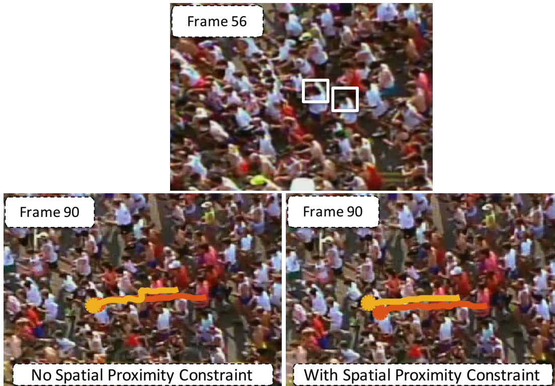
Figure 1.8: This figure aim to motivate the spatial proximity constraint used in our formulation. The top figure shows the two targets with very similar appearance. The bottom figures demonstrate the tracking results of our method, with and without proximity constraint. As can be seen when no spatial proximity constraint is used, the tracker gets confused and track of one target jumps to the near by one with similar appearance and motion. However, we are able to correctly track the two targets when we use the spatial proximity constraint as shown in bottom right figure.
