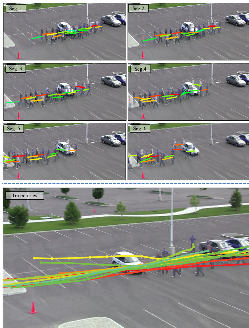
Figure 3.6: Top: The mid-level tracklets of six sample consecutive segments from Parking Lot sequence. Bottom: The trajectories resulting from associating mid-level tracklets of all the segments.
