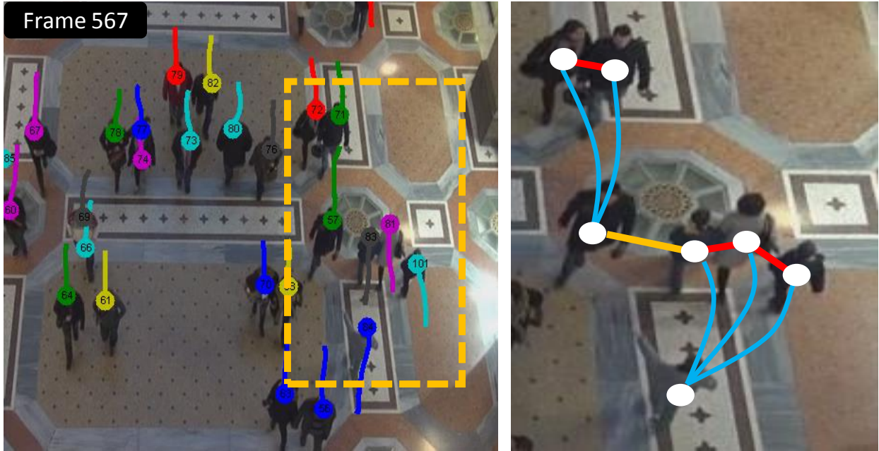
Figure 1.9: This figure is a graph illustration of the contextual constraints used in our formulation. The figure on the left shows the tracks and the figure on the right shows the constraints between the targets in yellow box. Each target is a node in the graph and all targets are connected with an edge. In practice there is a connection between every pair of targets but here for simplicity we are showing only some of the connections. The figure illustrates two groups walking in opposite directions as well as two individuals. Each edge is assigned a different cost depending on the grouping information and distance of targets from each other. The red edges that connect people in the same group encode the grouping and proximity constraints. The blue lines contain the neighborhood motion information and exist only between targets with coherent motion. The yellow edge only contains the spatial proximity information between two nearby targets.
