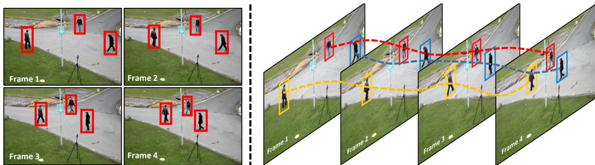
Figure 1.1: Multi-target tracking problem. Given a sequence of images, the task is to detect and construct the trajectory of each individual in the scene.
