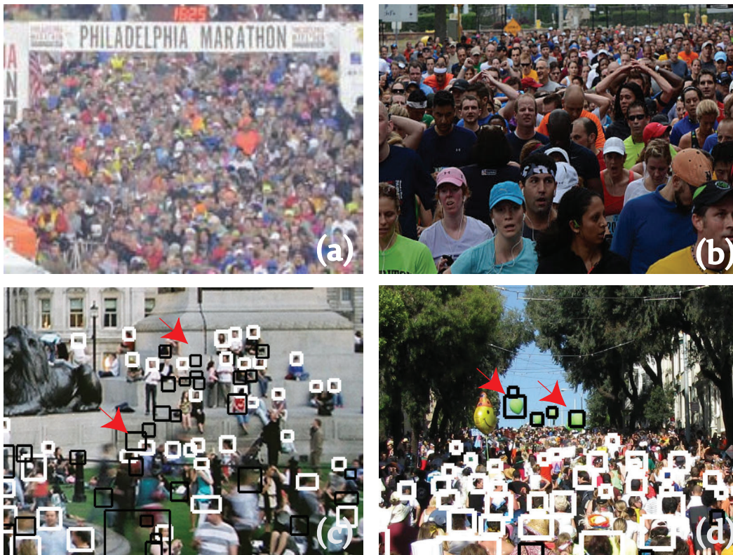
Figure 4.14: Failure Cases: (a) Blurring due to large distance from the camera in addition to small size due to perspective effects. (b) Camera position relative to humans in the scene may result in large number of occlusions where even the heads are partially occluded. (c) Hypersensitivity introduced due to priors caused by large number of high confidence detections in a low density region. (d) High-confidence false positives at the boundary of crowd may results in incorrect initialization of priors. In (c) and (d), true positives are shown with white, while false positives are shown in black.
