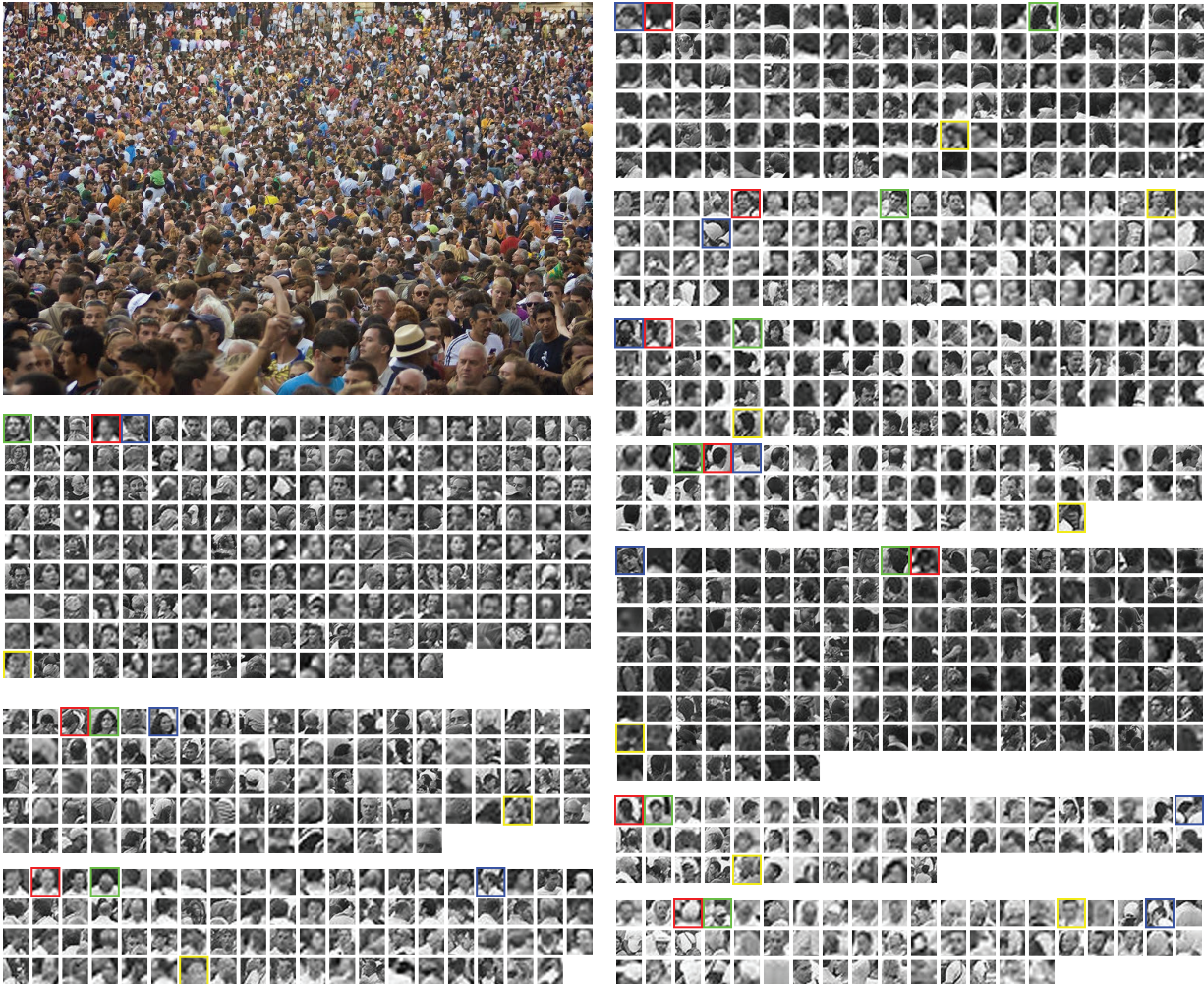
Figure 3.12: This figure shows the intermediate steps for discovering representative detection hypotheses. Each group of patches represents one cluster where the cluster center (mean) is marked with yellow box, while the top three representative patches are shown with red, green and blue, respectively.
