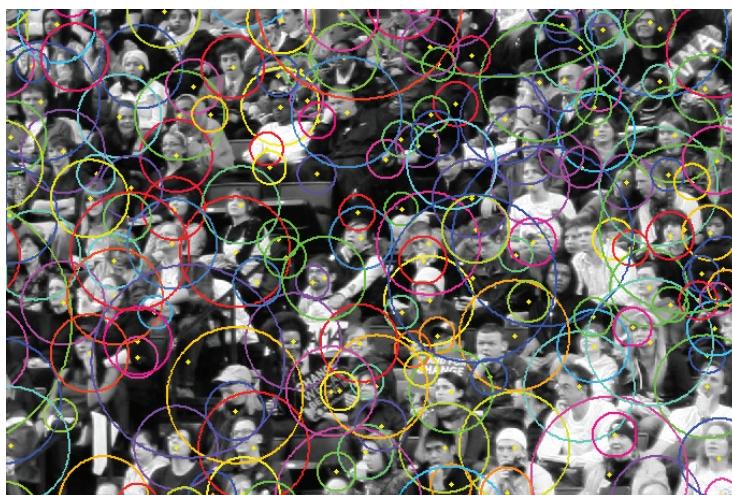
Figure 3.13: This image shows the Special Ordered Set (SOS) Type 1 constraints that are used during final selection of hypotheses. Each hypothesis (shown with yellow dot) enforces a constraint in its neighborhood (shown with colored circle) so that only one hypothesis is output by the algorithm at that location.
