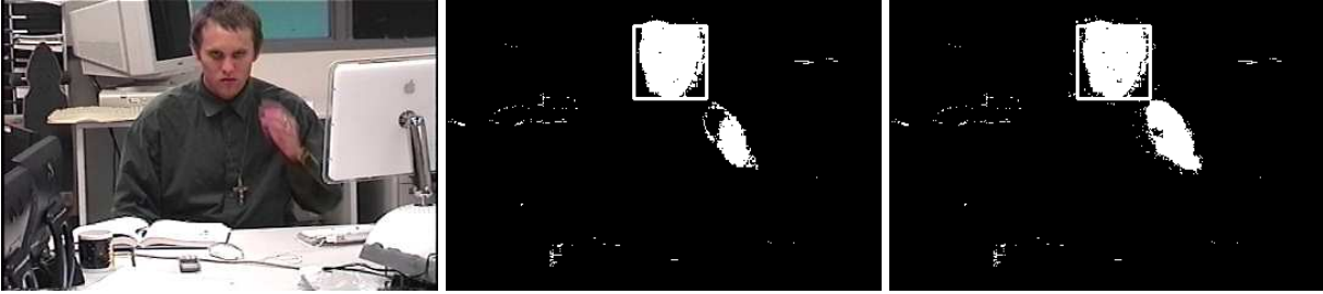
Figure 3.5: This figure shows how an incorrect result in one zoom can be used to correct future bad segmentations. Column 1 shows the input image. Column 2 shows the segmentation using the incomplete color model. This figure is the same as Figure 3.3 (column one, row three). Column 3 shows the segmentation of the same image after the notification and update process. This update of the color model allows for much better segmentation of the hand. This is an interesting consequence of the multizoom cooperation among cameras.
