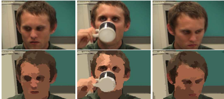
Figure 4.15: First row: Sequence showing person drinking from a mug. Second row: Mean shift segmentation performed on the above three frames. The idea of this feature is to count the number of segments in each given region. Here the region is the whole image.
