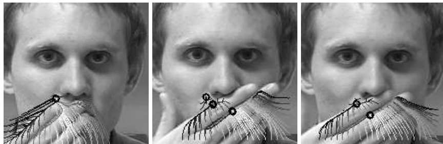
Figure 3.32: The hand region is shown with the channel lines superimposed on it. These channel lines are the ones that varied most from the previous location's model. A convex hull algorithm could be used to fill in this hand region.
