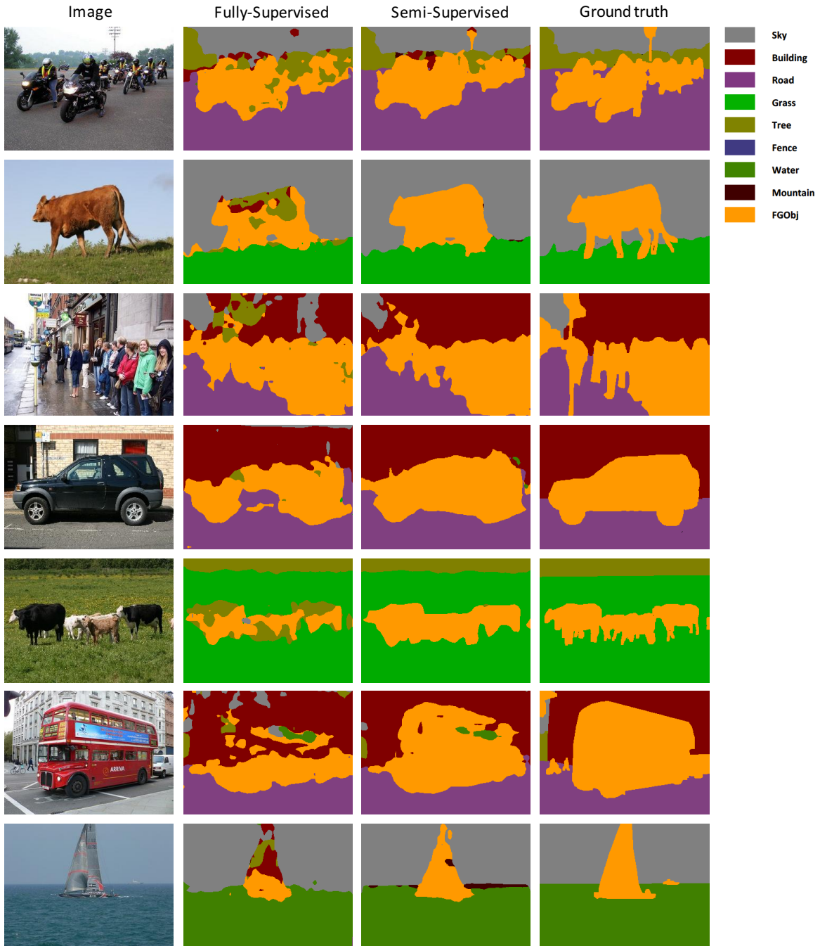
Figure 6.10: Qualitative results on StanfordBG dataset, using unlabeled data results in more accurate semantic segmentation, unlikely classes in the image are removed in semi-supervised approach.
