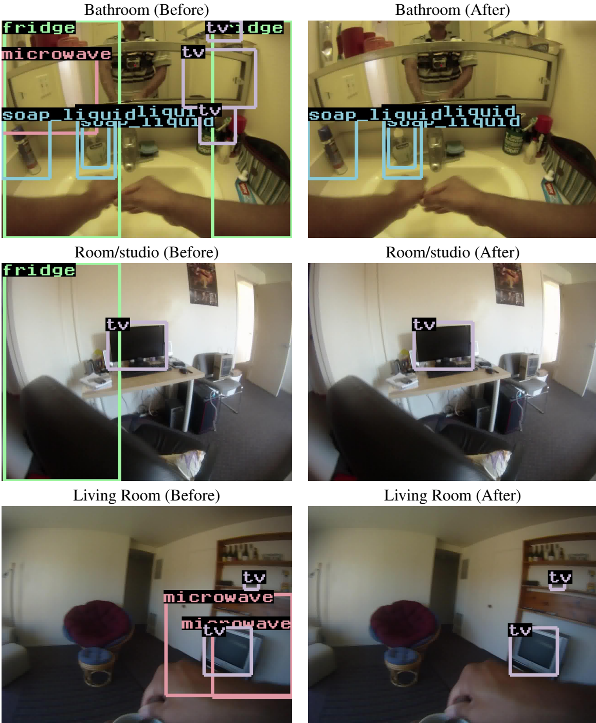
Figure 5.5: Qualitative results of the object detection before and after re-scoring the detections based on the scene. Many false positives are removed after the proposed re-scoring.
