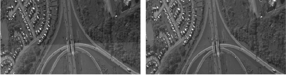
Figure 4.8: This figure shows the results of multi-camera intensity equalization. Notice the seam in the image on the left which is not visible in the equalized image on the right.
