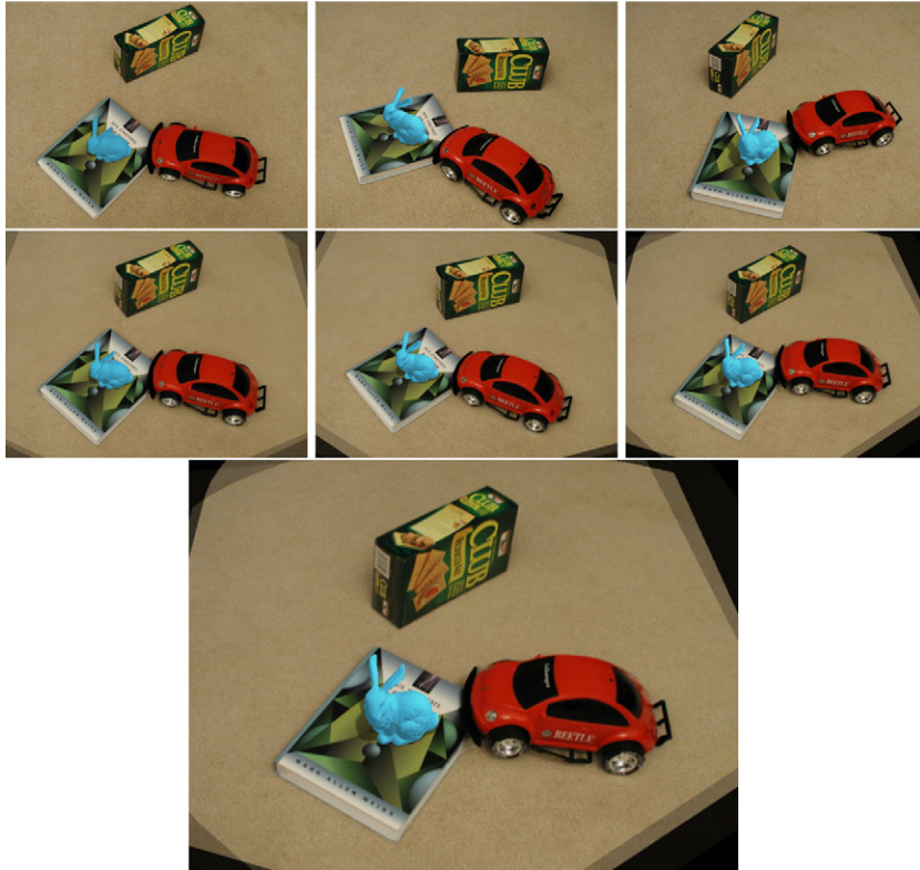
Fig. 8. Augmenting 3D object in tri-view morphing. The first row shows three original images with the augmented object (“Bunny” model from Stanford University). The 3D model is accurately augmented on the top of the book. The second row shows that a series of synthesized virtual views with the augmented object can maintain geometric correctness in the morphing procedure. We also generate the shadow of model and cast it on the book by assuming a light source. The bottom row shows the detail of one synthetic image.
