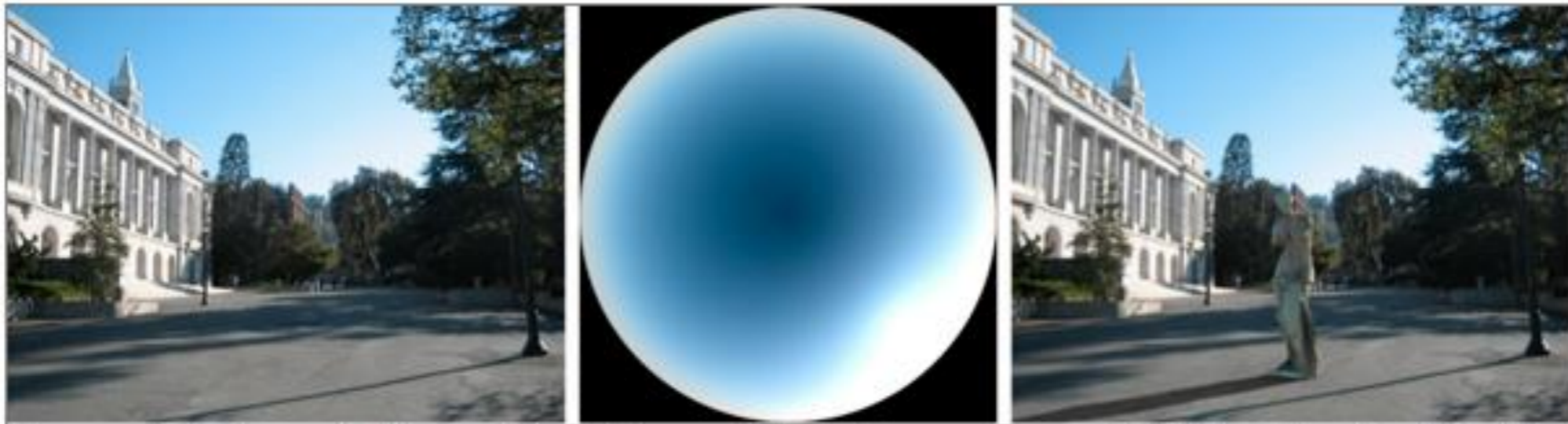
From a single image (left), we estimate the most likely sky appearance (middle) and insert a 3-D object (right). Illumination estimation was done entirely automatically.
