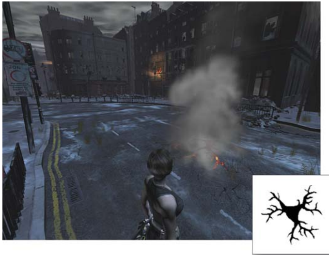
Figure 30-5. Smoke Rises from a Crack in the Ground in the Game Hellgate: London Inset: A slice from the obstacle texture that was used to block the smoke; white texels indicate an obstacle, and black texels indicate open space.
