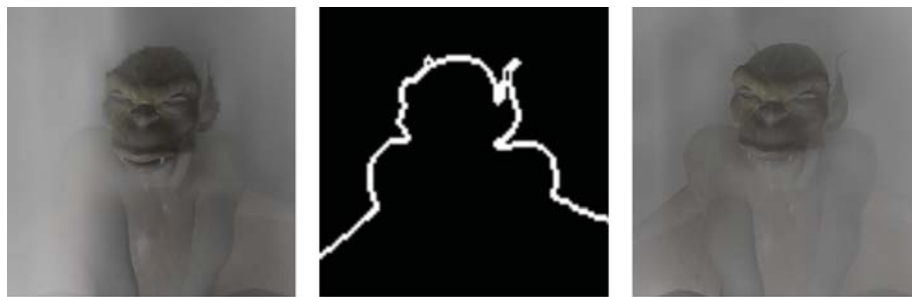
Figure 30-22. Fixing Artifacts Introduced by Low-Resolution Off-Screen Rendering Left: Ray marching at a low resolution and upsampling can cause artifacts near sharp silhouettes. Center: Detecting these features and rendering the corresponding fragments at higher resolution. Right: The resulting artifact-free image.
