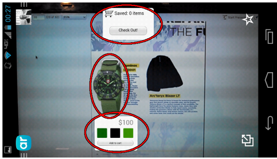
Figure 5: A Layar channel running on a scanned magazine page. The AR objects are circled. Clicking any color below the 3D watch model changes its color. The user can also add the watch to his or her shopping cart.
