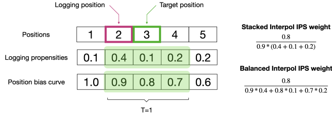
Figure 1: Illustration of the importance-weight computation for the stacked and balanced versions of Interpol , for the banded window system with T = 1 (green region). The target and logging policies place an item at position 3 and 2 respectively. For stacked Interpol , we compute the probability that the logging policy placed the item inside the window corresponding to the rank assigned by the target policy. For balanced Interpol , we compute the probability that the item was seen by the user in the window under the logging policy.
