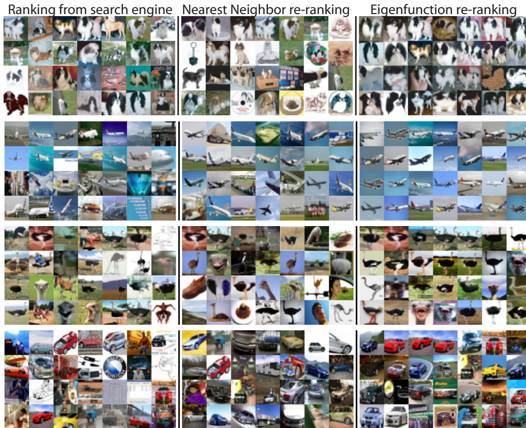
Figure 6: Re-ranking images from 4 keywords in an 80 million image dataset, using 3 labeled pairs for each keyword. Rows from top: “Japanese spaniel”, “airbus”, “ostrich”, “auto”. From L to R, the columns show the original image order, results of nearest-neighbors and the results of our eigenfunction approach. By regularizing the solution using eigenfunctions computed from all 80 million images, our semi-supervised scheme outperforms the purely supervised method.
