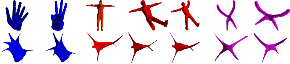
Fig. 2. Spectral embeddings (bottom row) of some articulated 3D shapes (top row) from the McGill shape database. The embeddings are constructed using the second, third, and fourth eigenvectors. The ignoring of the first eigenvector is explained in Section 5.
