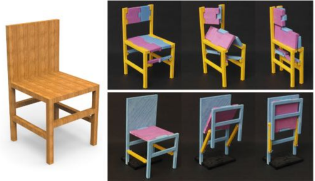
Figure 1: Two automatic foldabilizations of a chair with respect to two folding directions. Shown on the right are fabrication results produced by a MakerBot Replicator II 3D printer. Folding is possible by adding hinges, shrinking parts (chair back in the top row), or allowing slanting or shearing, leading to less hinges and better structural soundness (bottom right). The foldable chair in the top row resembles the Stitch Chair by the designer Adam Goodrum.
