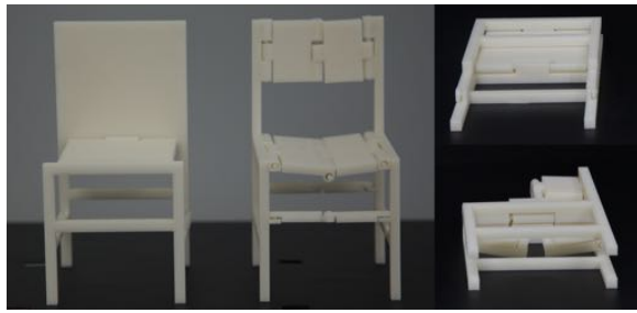
Figure 24: Photographs showing two chairs in their unfolded configurations (left); each of them is fabricated in the folded state (right) using an FDM printer with dissolvable support material.
