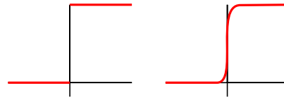
Figure 3: Support distance functions (SDFs) to identify front-facing planes. The left-hand function is discontinuous, and cannot be used as an SDF. The right-hand function is an acceptable substitute.
