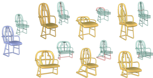
Figure 9: Six mutations on the chair model on the left. Controllers undergone mutations are highlighted in red. Structure optimization of the controllers ensures coherence of the resulting models.
