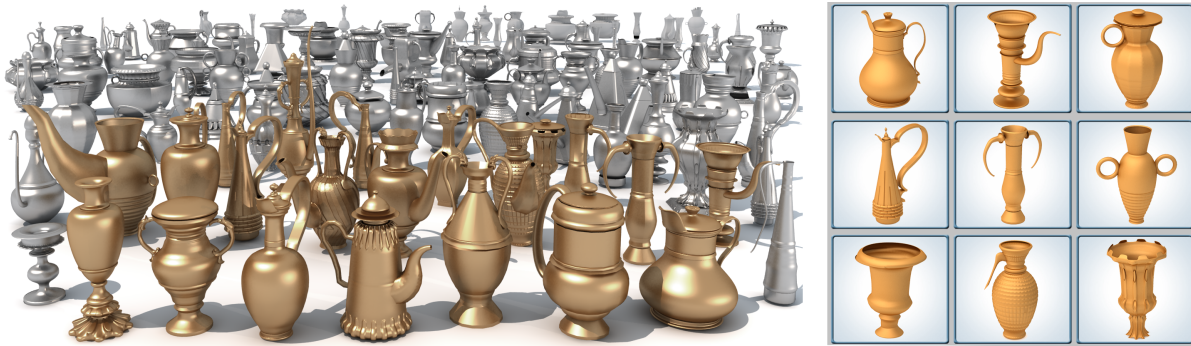
Figure 2: The evolving population (left) consists of a diverse background set (in gray) and a fit foreground set (in gold). The gallery of shapes that is presented to the user is illustrated on the right, which consists of shapes taken from the foreground set.
