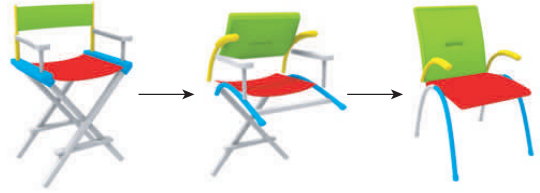
Fig. 4. An in-between shape obtained via a structure-preserving deformation [Alhashim et al. 2015] is not plausible. Yet, its associated energy is relatively low due to the strong effort in the structure preservation.
