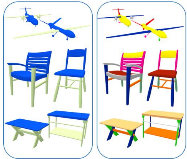
Fig. 1. Shape correspondences, derived by our hierarchical search, between 3D shapes exhibiting significant geometry and topology variations. Results at two granularity levels are shown. The topology-varying part matchings are computed where the core evaluation mechanism only performs shape recognition with respect to a shape repository. Matched parts share the same color; unmatched parts are in gray.
