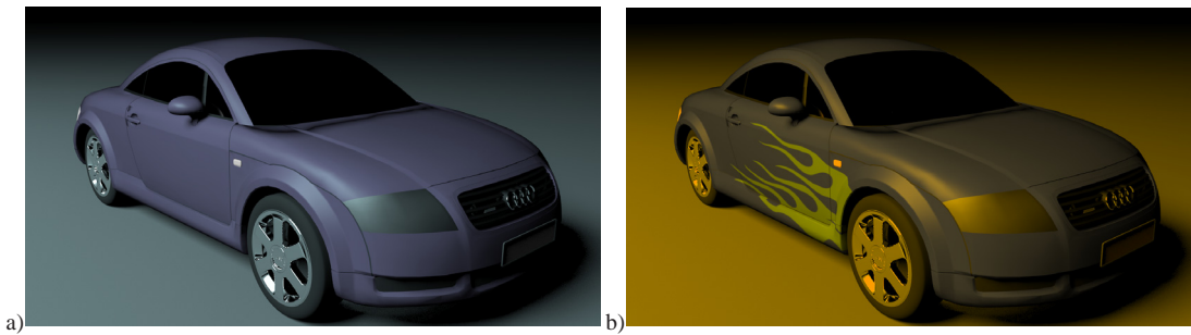
Fig. 5. Car model rendered with PBRT. (a) The spectral materials used in the texture are metameric under daylight D65, resulting in a monochrome appearance. (b) Changing the illumination spectrum to that of a high pressure sodium lamp, as used in street lighting, breaks apart the metamerism and reveals additional visual information.
