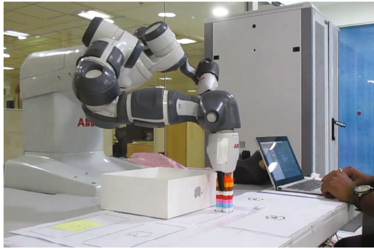
FIGURE 4 Set-up of the experiment: The robot is set up next to the programming environment in front of our participants. In the task shown here, users are instructed to pick up the lego-like object and place it into the white box.
