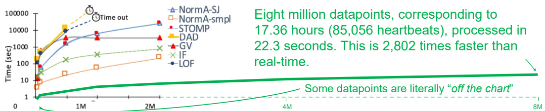
Fig. 23 (Most of this figure is taken from [4] with permission, only the green elements are new). The scalability of various algorithms on increasing large subsets of a long ECG trace. All algorithms except DAMP are limited to the first 2M data points by [4]. Note that the Y-axis is logarithmic.
