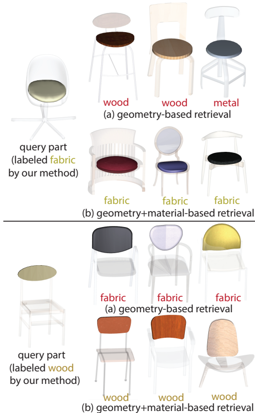
Figure 6: Given a query (untextured) part of a 3D shape and its material label predicted by our method, we can search for geometrically similar parts by considering (a) geometric descriptors alone, or (b) geometric descriptors together with material labels. Note that we discard any retrieved parts that are near duplicates of the query parts to promote more diversity in the retrieved results.
