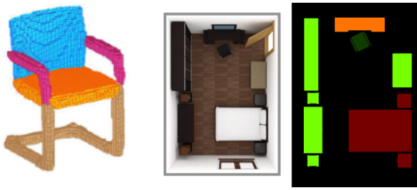
Figure 3: Representing 3D structure via segmented geometry. Left: representing the part structure of a 3D object by part-labeled voxels [WSH*18]. Right: Representing a 3D scene via a floor plan image with per-pixel object type labels [WSCR18].
