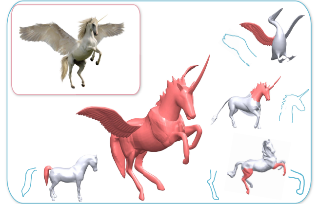
Figure 11: Example of image-driven part-based modeling. Given the image (on the top left corner), the user sketches the contours of the parts of the shape. Our method extract parts from the database. The user selects the parts and assembles the 3D shape (middle) in the image. The body part of the generated shape is segmented from an existing horse shape.
