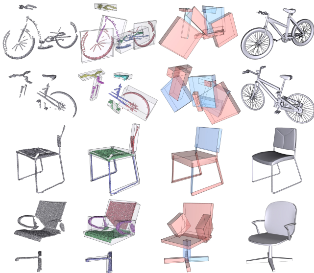
Fig. 18. Complete shapes reconstructed from noisy, incomplete point clouds using SCORES. Newly generated OBBs are marked in blue.
