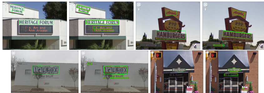
Fig. 11: For each pair of images, left: the original incomplete annotation, right: detection result of our model as well as the fully annotated ground truth. The fully annotated dataset provides oriented bounding box annotation. Green boxes represent our detected result which matches the ground truth. Yellow boxes represent the ground truth.
