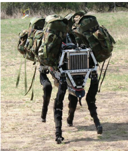
Big Dog™ robot was developed as a "mule" to traverse difficult terrain.
