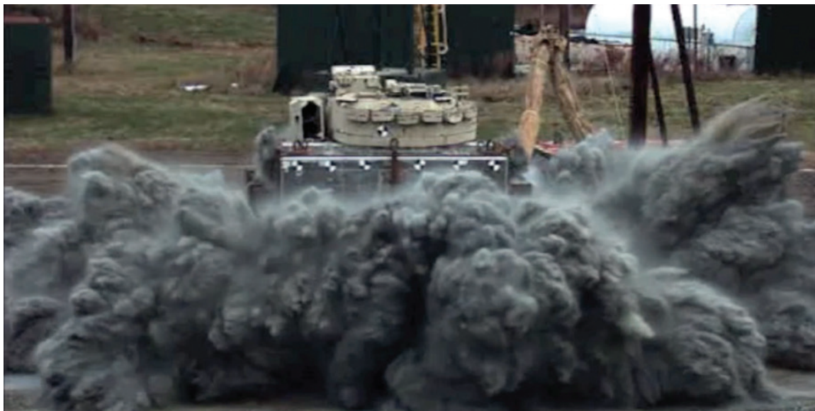
Underbody explosion test (10x over SOA) on a blast resistant vehicle integrated with a multi-level energy absorbing system allowing all of the occupants to survive with minimal injuries.
